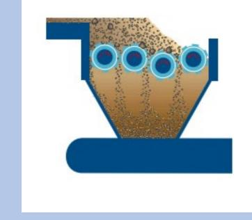
Sub-25 mm clinker falls through the gaps between the transport rollers, while the bigger lumps are conveyed forwards onto the crusher rollers. The first of these is the 'dropped roller', which sits slightly below the horizontal plane of the other rollers. This one rotates clockwise, while the final crusher roller rotates counter-clockwise, pulling the oversized clinker into the nip where it is crushed between the teeth of the cast wear segments.
